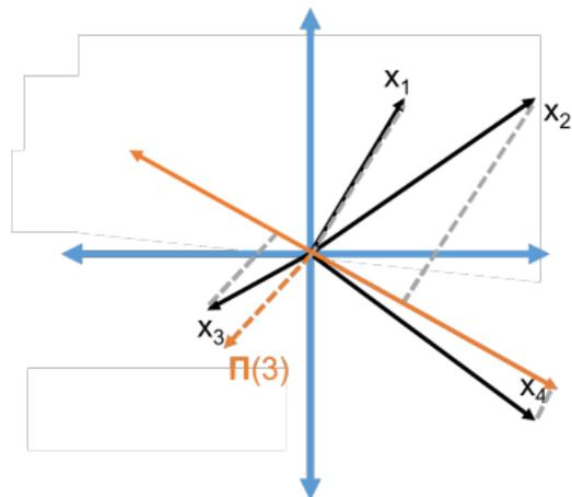
$x_1, \dots, x_n$ : original points ( $d$  dims.),  $\tilde{x}_1, \dots, \tilde{x}_n$ : compressed points ( $d' < d$  dims.),  $\mathbf{\Pi} \in \mathbb{R}^{d' \times d}$ : random projection (embedding function)
